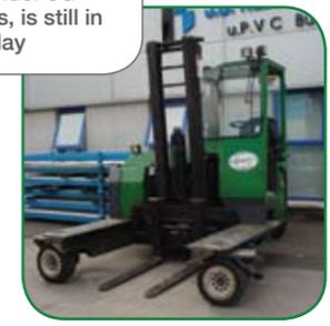
The Combilift fills a niche in the market for a versatile forklift for the safe and space saving handling of long loads in confined spaces
