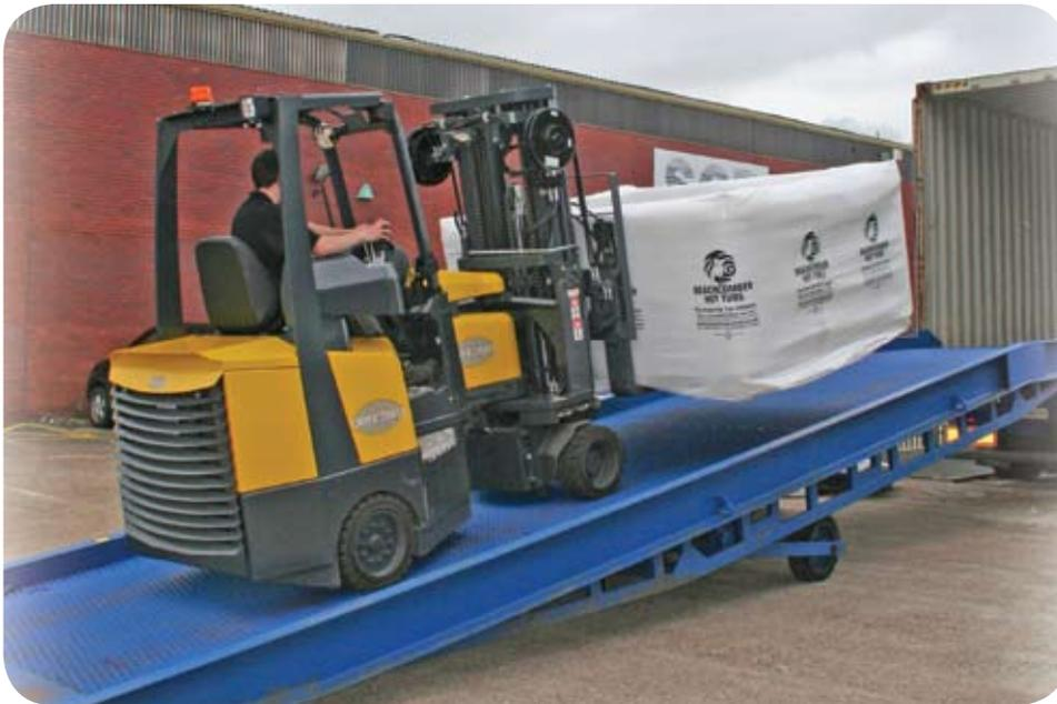
*Aisle-Master articulated trucks are wholly designed and manufactured in Ireland and enjoy an unrivalled reputation for quality and long life operation. They can work in aisles of just 1.75m, have capacities of up to 2.5 tonnes, lift heights of up to 15m, with a choice of AC electric or LPG power. A parts warranty of 5 years or 5,000 hours now offers even more peace of mind for users and underlines the extreme reliability of the range.*
