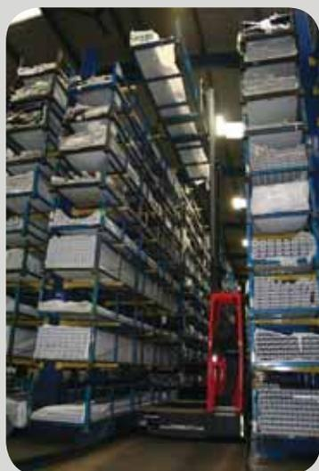
The ST's compact dimensions enable it to work in any existing racking designed for Hunslet operation
