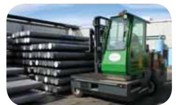
The 4-way SL series was developed following requests from conventional sideloader users for a more manoeuvrable truck able to provide better storage density and block stack whilst working in pre-existing aisle-widths. Combilift sideloaders are available with capacities from 4.5 - 6t, a wide range of options and a choice of front or rear cabs.
