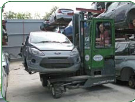
By replacing its rough terrain truck with a 4t capacity Combilift, Atkinson Car Dismantlers has more than doubled its storage capacity. Aisle-widths between storage bays in the yard have been reduced from 22ft to 13ft, freeing up space for a total of 275 cars compared with a previous tally of around 100.
