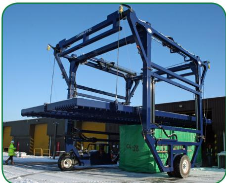
One of Combilift's largest capacity models to date - a 28t capacity Straddle Carrier (Combi-SC) - is now in operation at Caledonian Modular's site in Newark near Nottingham, ensuring much more efficient and safe transportation of finished modules from the manufacturing facilities to the storage yards.
