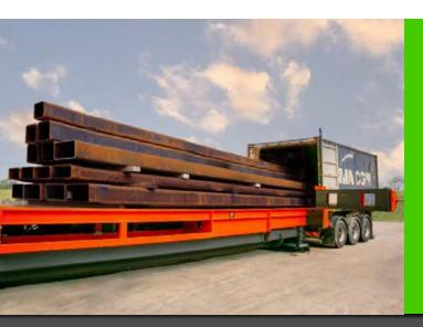
A cost-effective container loading solution that can load/unload a 40' container in as little as 6 minutes.
