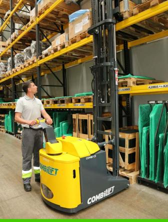
This pedestrian reach stacker can operate in the narrowest aisles of any truck of its type in the market.
